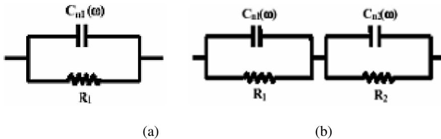
Figure 2. Equivalent circuits used for fitting experimental data.
