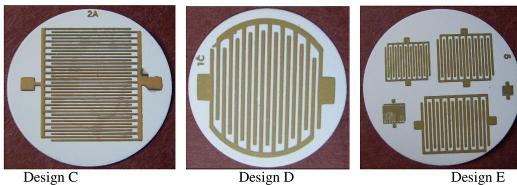
Figure 7. Images of three sensors fabricated on nano-porous nylon membrane with Si shadow masks, corresponding to design C, D, E. (All membranes are 25 mm in diameter.)
