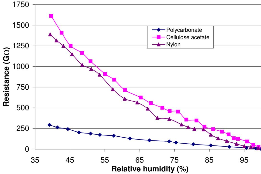
Figure 10. DC resistance vs. relative humidity for three design C devices fabricated on polycarbonate, cellulose acetate, and nylon membranes, respectively, at 25 C°.
