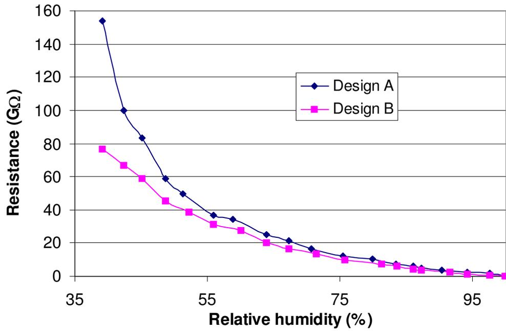
Figure 9. DC resistance vs. relative humidity for design A and B devices fabricated on polycarbonate membranes at 25 C°.
