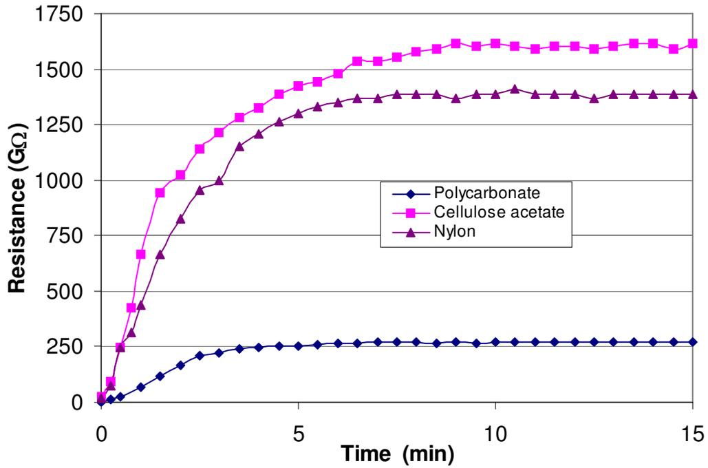
Figure 11. Time response of the three design C devices (in figure 10) when they were taken out from a 100% to 39% relative humidity environment at 25 C°.
