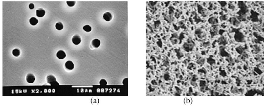
Figure 1. Micrographs of the two nano-porous sensing materials: (a) polycarbonate and (b) polyester membranes.
