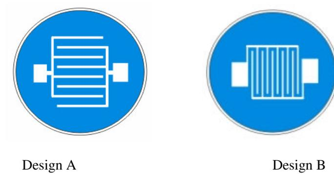
Figure 3. Design A and design B of humidity sensors. (Diameters are 25 mm for both designs.)
