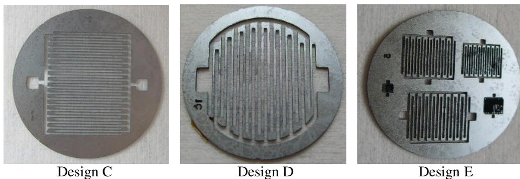
Figure 6. Si shadow masks fabricated by deep RIE etching of Si with electrode patterns corresponding to design C, D, E. (All Si shadow masks are 26 mm in diameter.)
