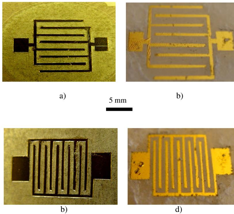
Figure 5. Images of the two humidity sensors fabricated on polycarbonate membranes with adhesive paper shadow masks. a). Design A sensor after sputtering before removing the paper mask. b). Design A device after removing the paper mask. c) and d). Same as a) and b) but for a design B sensor.
