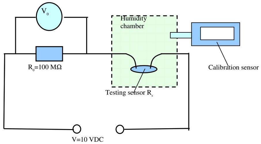
Figure 8. Test setup for the humidity sensors.
