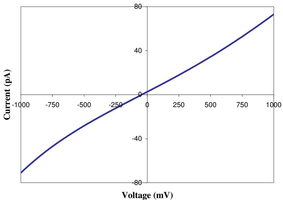
Figure 12. I-V curve of a design D sensor fabricated on polycarbonate membrane.
