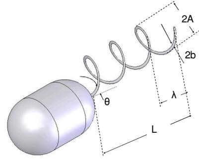
Fig. 2. Schematic of the swimming microrobot propelled by flagellar motion
