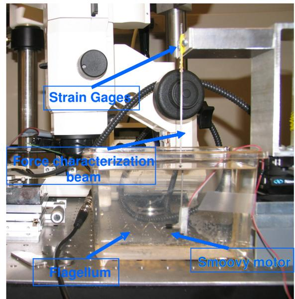
Fig. 4. Force measurement system
