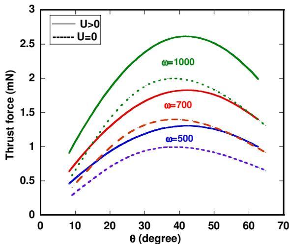
Fig 3. Thrust force as a function of  $\theta$  for different angular velocity of the flagellum
