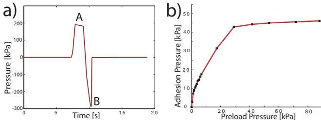
Fig. 2. Force vs. time data plot for a single adhesion test (a) and performance curve for V10 on Acrylic (b).
