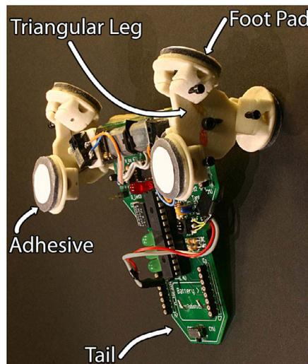
Fig. 1. Photograph of prototype Tri-Foot Waalbot climbing a  $90^\circ$  (vertical) surface.
