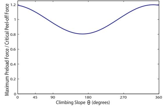
Fig. 6. Plot of preload/peeling force ratio for various values of slope angle  $\theta$  generated from (1).
