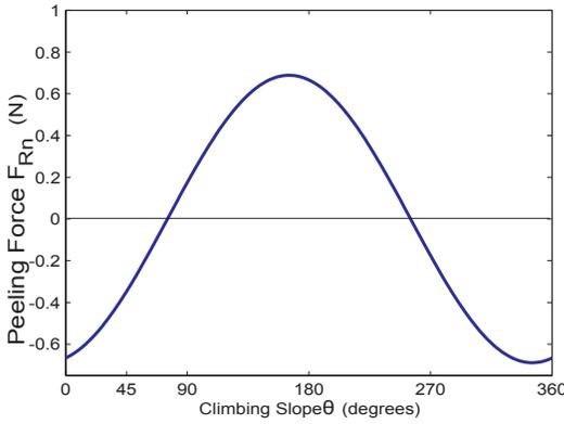
Fig. 7. Plot of the minimum normal peeling force which the adhesives must overcome for the robot to climb a slope of angle  $\theta$ .
