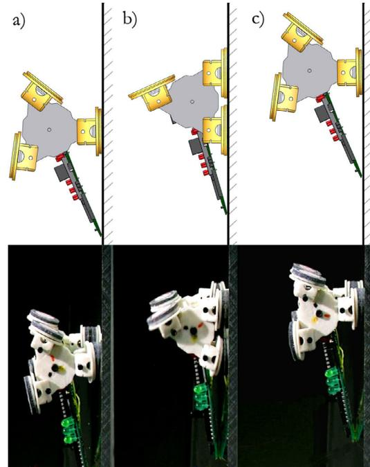
Fig. 4. Schematic side view of Waalbot climbing a vertical surface (top) and still photo frames from a video of the Waalbot prototype performing the same actions (bottom).
