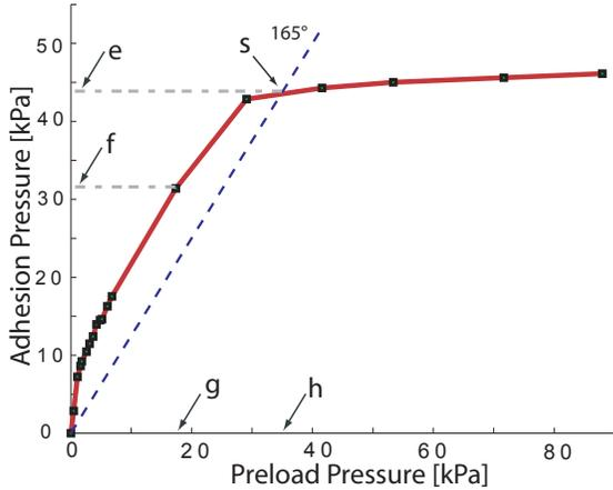
Fig. 9. Performance plot showing the minimum adhesion requirement (f), minimum safe preload (g), and steady state operating points (s, e, and h) for climbing a surface of  $\theta = 165^\circ$ .
