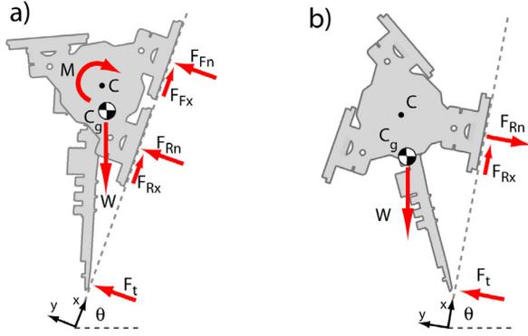
Fig. 5. Free body diagrams showing the forces during a forward step where the front foot is pressed against the surface and the rear foot is peeled (left), and in the configuration in which the robot experiences the highest peeling force while climbing (right).
