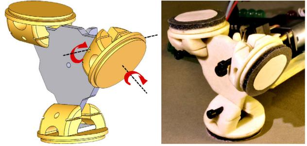
Fig. 3. CAD model of the Tri-Foot design (left) and assembled prototype components (right). Each foot pad has two degrees of freedom enabling climbing and steering.
