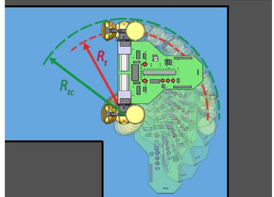
Fig. 10. Waalbot's small turning radius ( $R_t$ ) and turning circle radius ( $R_{tc}$ ) let it climb around obstacles and operate in narrow corridors with sharp bends (top).
