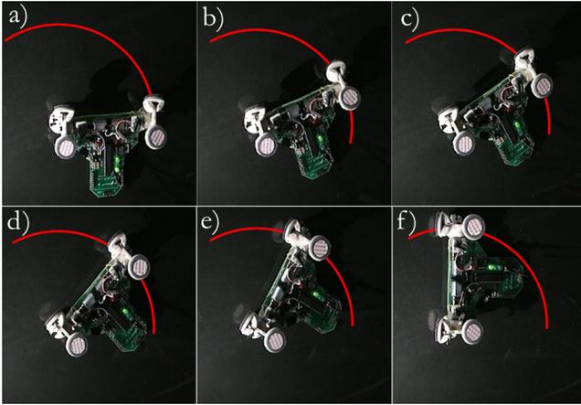
Fig. 11. Still frames from a video showing a Waalbot prototype turning while climbing on a vertical acrylic surface. The prototype turns  $90^\circ$  (line overlaid) in six steps (bottom a-f).
