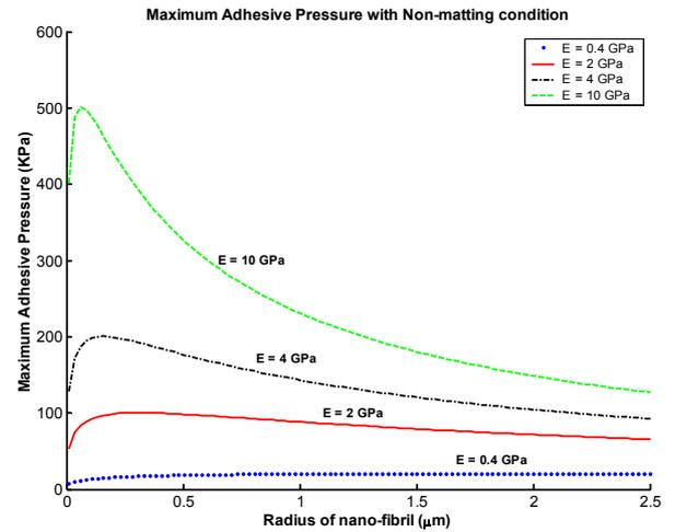
Fig. 6: Maximum adhesive pressure as a function fiber radius using the non-matting condition and van der Waals force model
