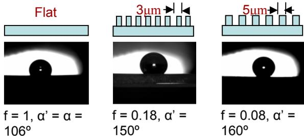
Fig.12: Experimental results from contact angle measurements on PDMS fibrillar adhesives: flat surface (leftmost), 3  $\mu\text{m}$  diameter fibers (middle), and 5  $\mu\text{m}$  diameter fibers (rightmost)
