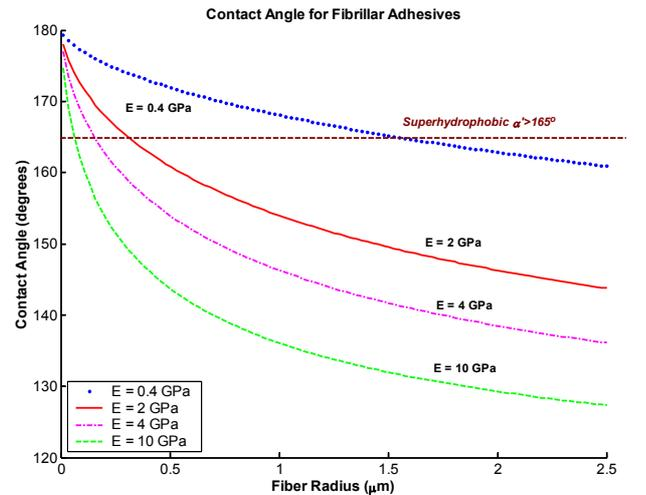
Fig.11: Contact angle for fibrillar adhesive using Cassie's equation
