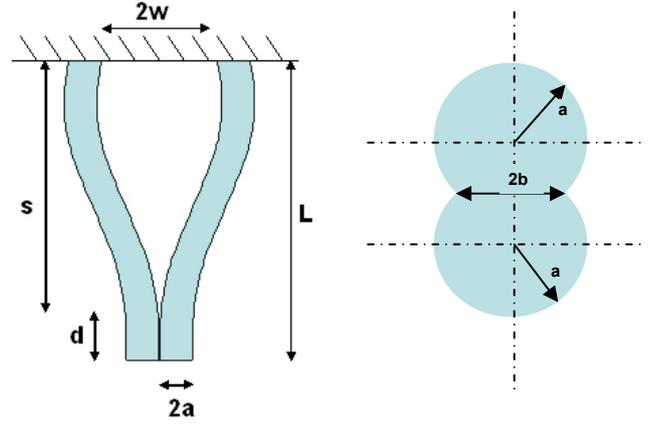
Fig. 5: Matted fiber model to determine minimum spacing between fibers
