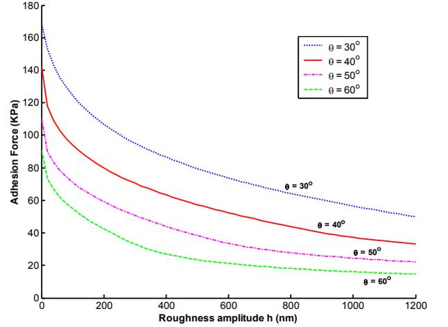
Fig.9: Adhesion force as determined from the surface roughness and fiber orientation
