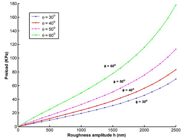
Fig. 8: Preload for good contact as determined from the surface roughness and fiber orientation
