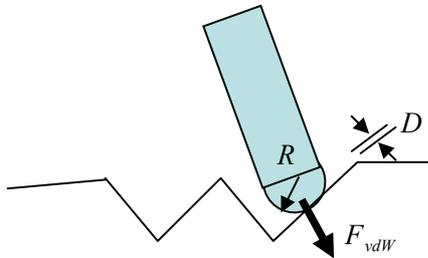
Fig. 3: Fiber adhesion through van der Waals force
