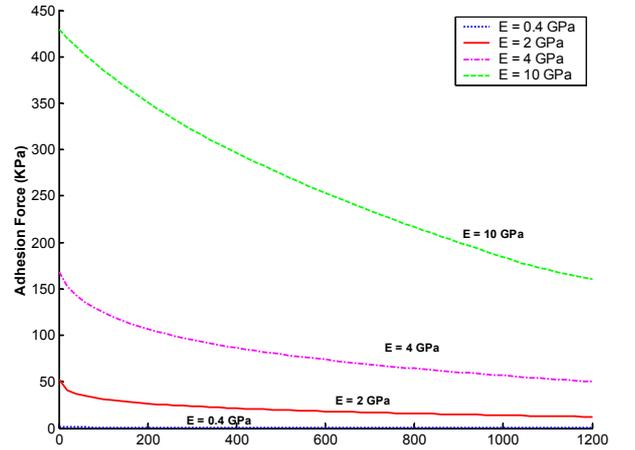
Fig.10: Adhesion force as determined from the surface roughness and fiber elastic modulus
