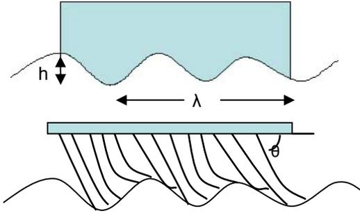
Fig. 7: Rough surface adaptation through fibrillar structure
