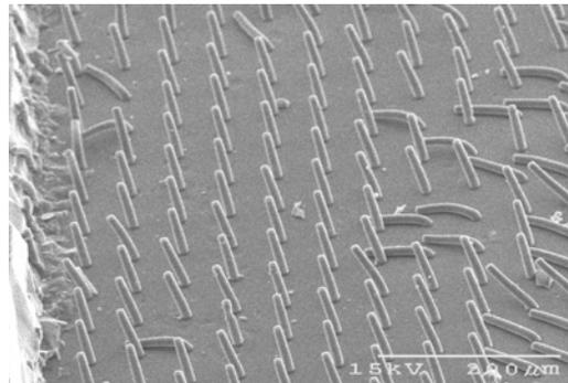
Fig. 1: SEM image of the polymer fibrillar adhesive fabricated at the NanoRobotics Laboratory, CMU
