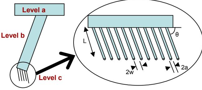
Fig. 2: Multiple levels of compliance in gecko-foot hairs
