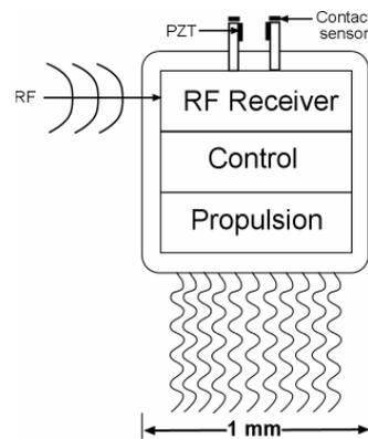
Figure 1: Overall design of swimming micro-robot.
