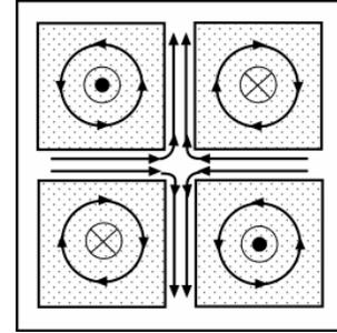
Figure 7: Independent rotation of four plates enables maneuverability.
