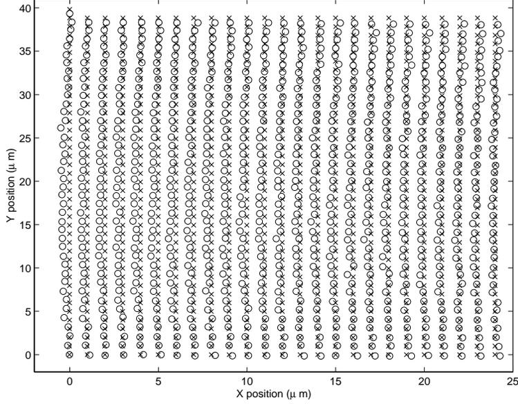
Figure 9: Controlled x-y scanning of the Stage I, and automatic tracking of the selected particle ('x' stands for the stage x-y position, and 'o' does for the transformed particle center position) for the calibration of the image to stage coordinate frame transformation.
