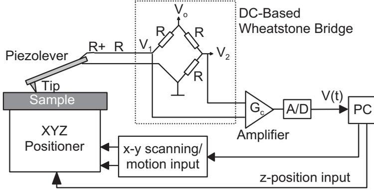
Figure 5: AFM with piezoresistive cantilever and electronic deflection detection system.
