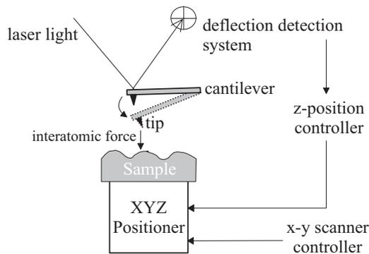
Figure 3: The basic structure of a conventional AFM.
