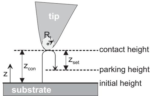
Figure 7: Parking height setting for the tip.
