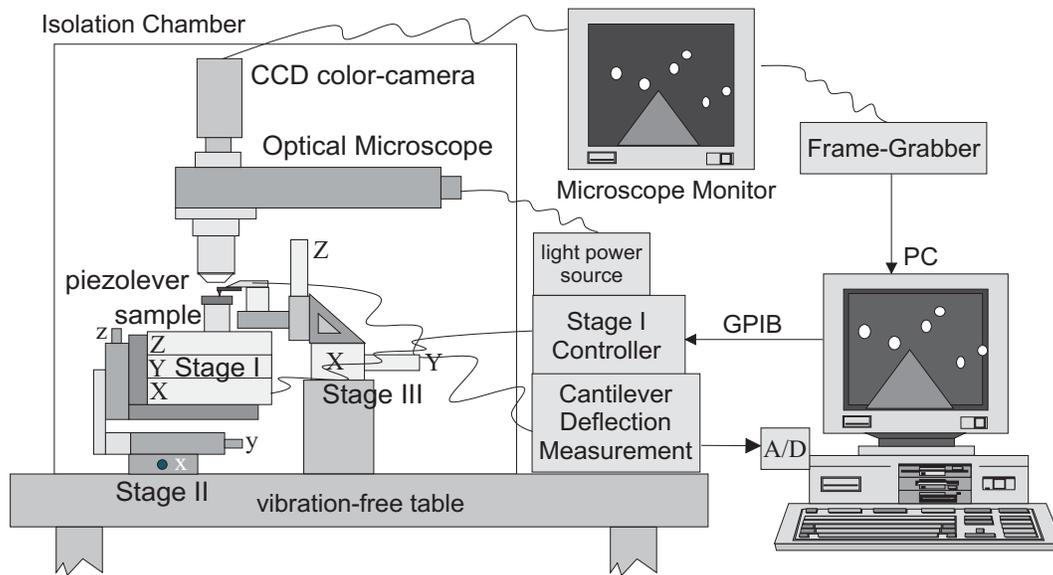
Figure 2: Overall system setup for the fine particle assembly.
