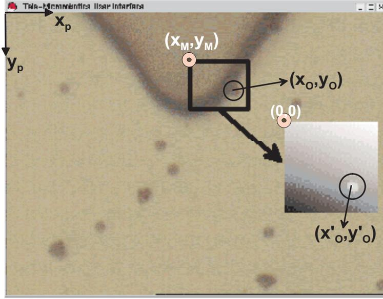
Figure 8: Automatic tip center position calibration using the tapping mode AFM imaging and selecting a  $1 \mu\text{m}$  size particle close to the end of the cantilever end with a known center position in the image coordinates.
