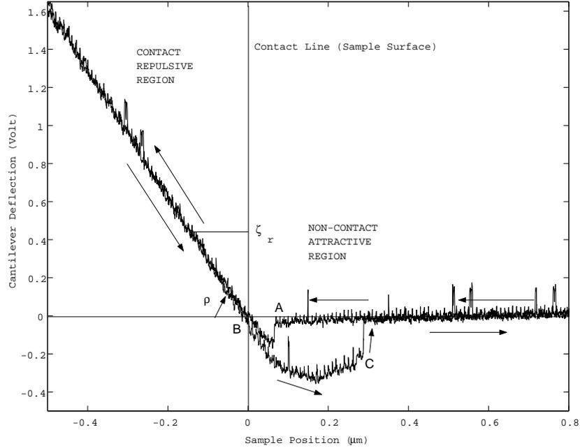
Figure 4: The typical cantilever deflection, i.e. inter-atomic force, and sample position relation for a silicon sample (experimental).
