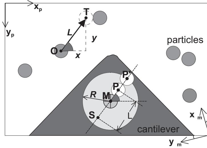
Figure 6: Automatic pushing or pulling operation, and image and positioner coordinates.
