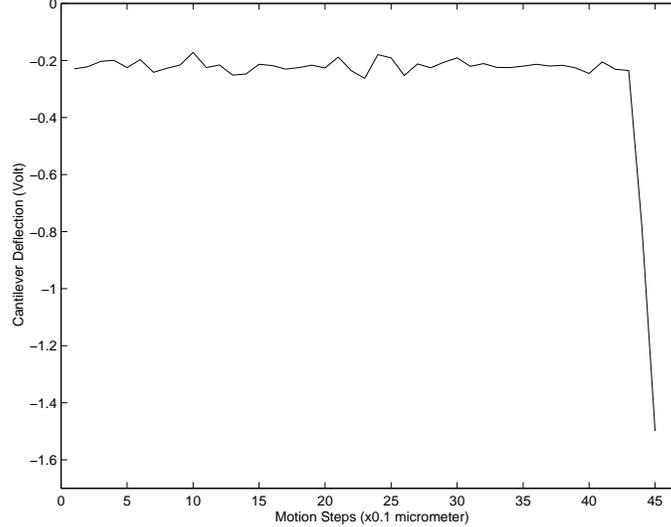
Figure 11: The cantilever deflection during automatic contact detection.
