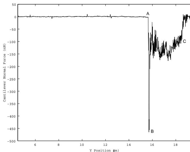
Figure 14: Measured cantilever deflection force during pushing the  $1\mu\text{m}$  size particle ('-' force values stand for a repulsive/compressive force).
