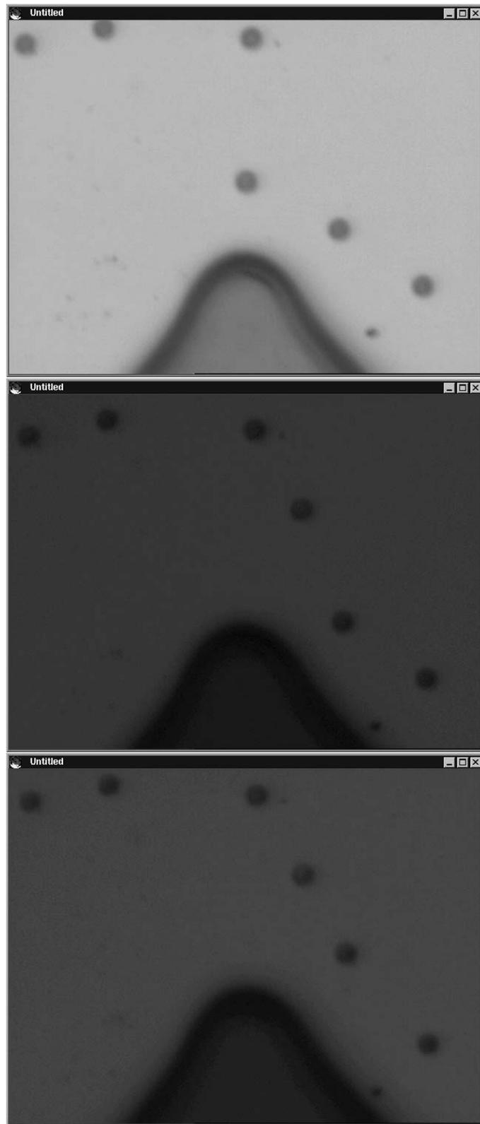
Figure 12: Positioning two particles with  $2 \mu m$  size: initial positions (uppermost), first pushing (middle), and second pushing (lowermost).
