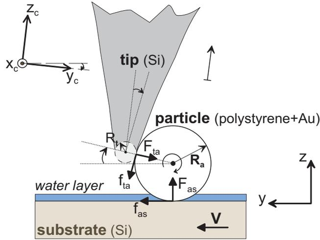
Figure 1: Positioning of the fine particles using the AFM tip as the contact pushing/pulling manipulator.
