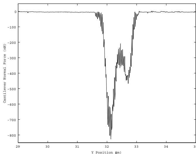
Figure 15: The tip and particle can lose the contact shortly after the initial push due to the pushing direction misalignment.
