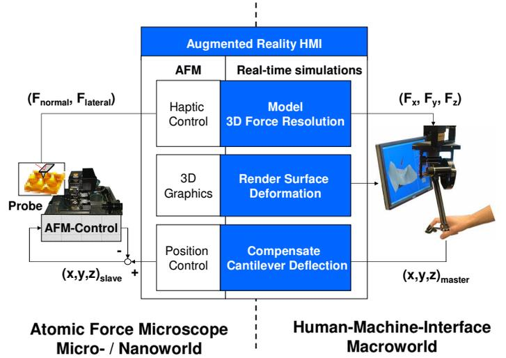
Figure 2. System concept: Sensed and simulated information are blended in real-time.
