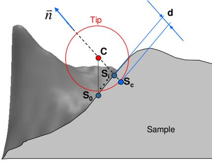
Figure 3. Collision detection yields normal direction  $n$  and indentation depth  $d$ .
