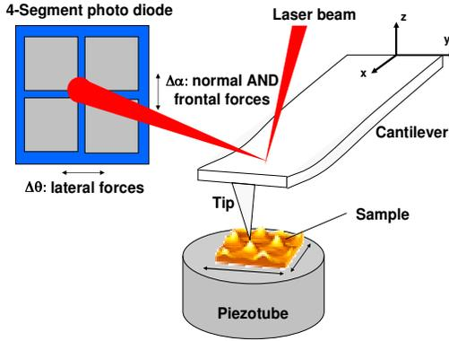
Figure 1. AFM force sensing: frontal and normal forces are measured in a coupled way, while lateral forces are measured separately. Therefore, decoupled 3D-force feedback is not possible.
