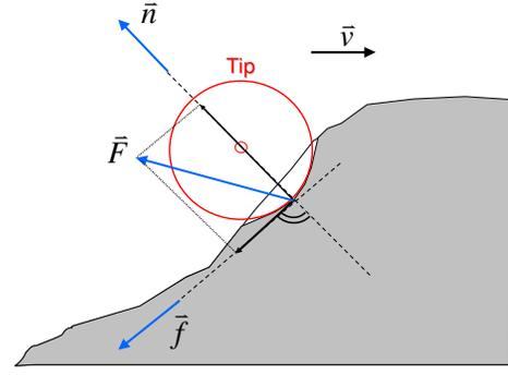
Figure 5. Geometry of the tip-sample contact.
