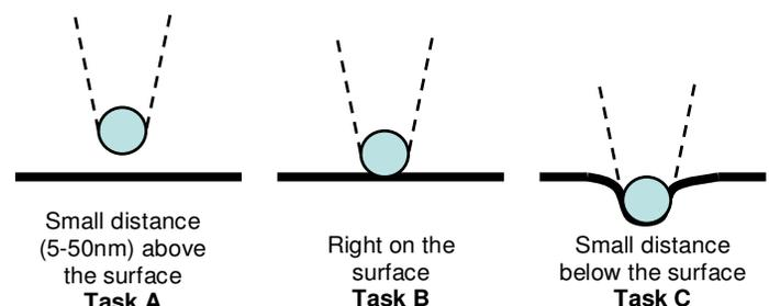
Figure 9. Experiment tasks (the sphere represents the AFM tip).
