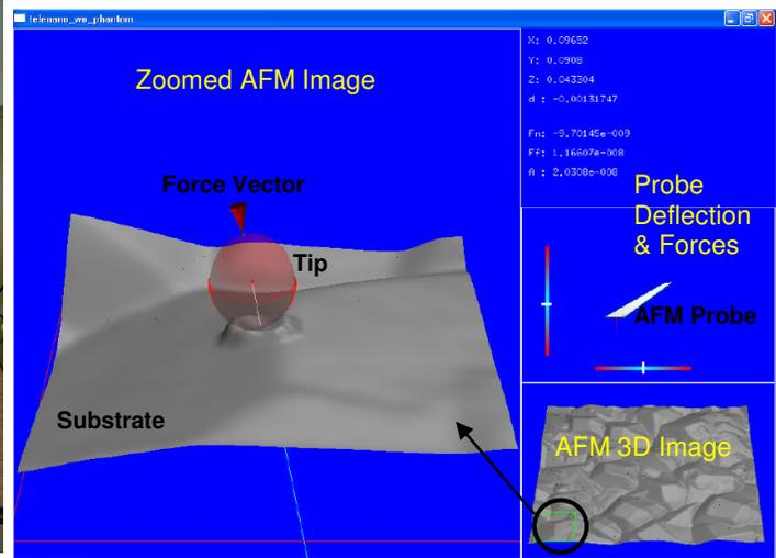
Figure 8. Snapshot of the implemented graphical user interface: left window shows the 3D real-time probe tip, zoomed AFM image of the surface, and nanoforces; right-bottom window displays the overall 3D AFM surface topography; right-middle window displays the AFM cantilever deflections; right-top window shows the real-time data of 3D forces and AFM tip position.
